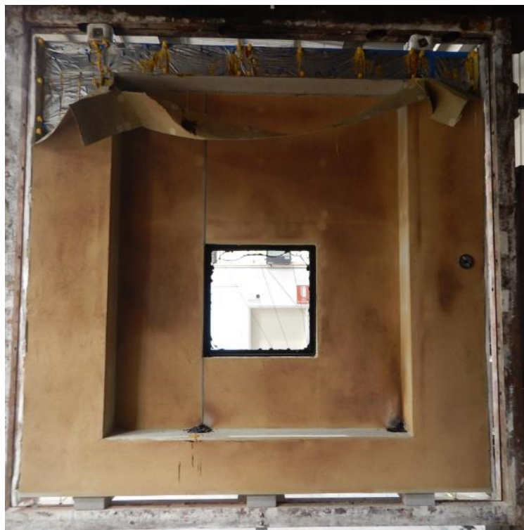
Figure 17 Exposed face of the specimen at the end of the bush fire test
