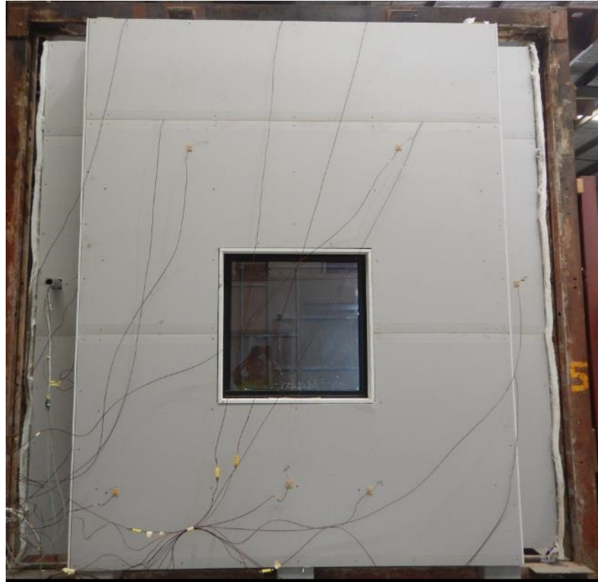
Figure 14 Unexposed face of specimen before the start of the bush fire test
