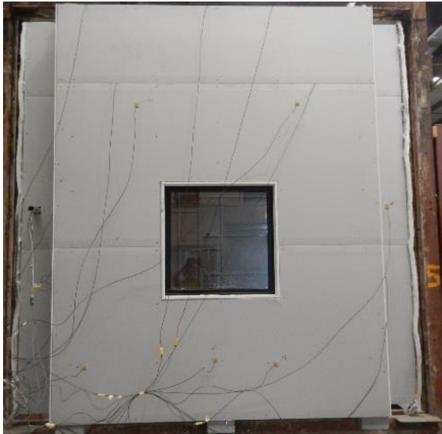
Figure 16 Unexposed face of specimen at the end of the bush fire test
