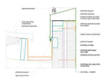
In all cases the StateWall® External Wall Cladding System must only be installed in accordance with the Technical Manual on steel or timber wall framing with a maximum stud spacing of 600mm
